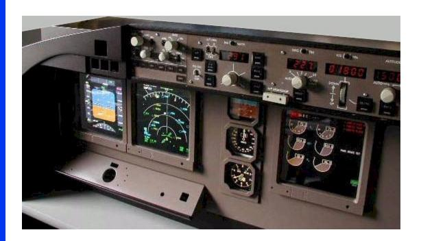
The Glass Cockpit Trainer (GCT) is a modular, portable, desktop solution to your transition training requirements. In addition to providing a complete Primary Flight Display (PFD) and Navigation Display (ND), the GCT also includes a fully functional FMC/CDU modeled after the Boeing/Smiths unit.
